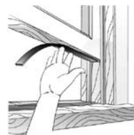
Open Cell Foam Tape installed on casement window.
